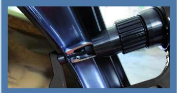
A special transmission delivers high torque at reduced RPM in order to prevent overheating the carbide bits. This is done without the need to reduce incoming air pressure which would result in the loss of torque.
